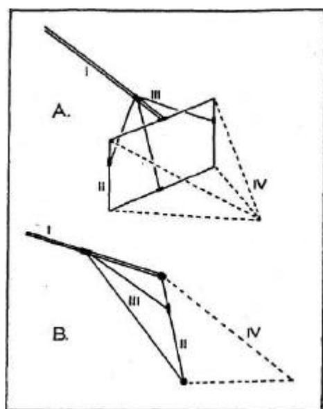
Fig. 2. Sampling net. The net was used to determine the type and average weight of prey eaten by the spoonbills. Sampling took place at the spots where foraging spoonbills were observed. A: 3- dimensional view of the net. B: Side view. I: Handling stick. II: Window frame (80 x 40 cm). III: Support rods. IV: net (5 mm mesh).
