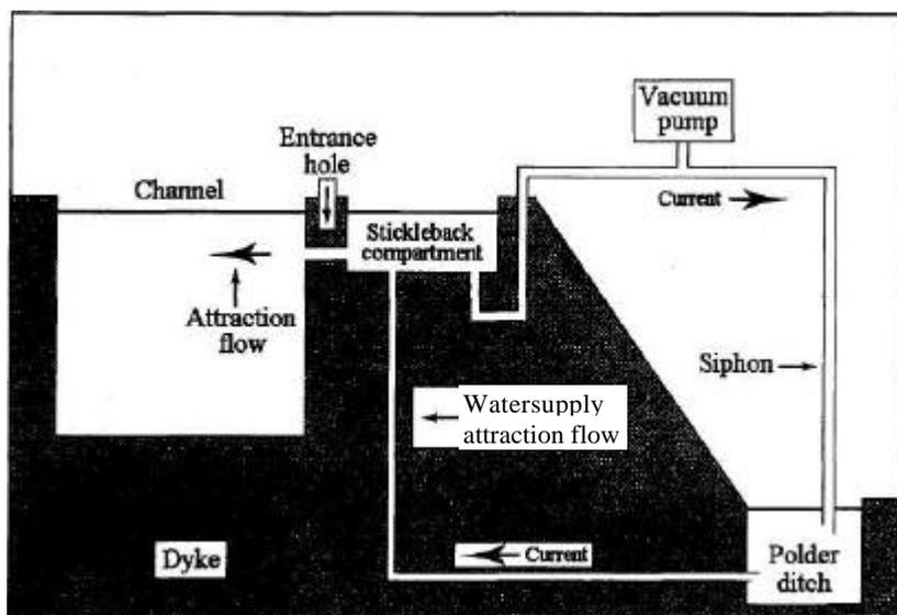
Fig. 9. Outline of the siphon fish ladder. The dyke is a barrier that separates the channel from the polder ditch, and so disables anadromous sticklebacks to migrate to spawning grounds. The siphon fish ladder is designed for this typical Dutch problem. For an explanation see the text.
