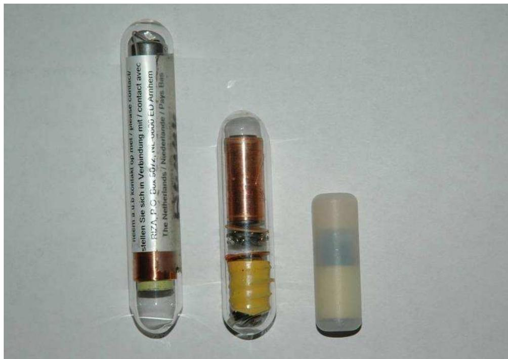
**Figure 1.** Different sizes of transponders used with the NEDAP TRAIL system®
